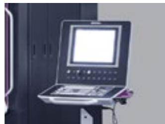
Moving control panel with 19" touch screen.
