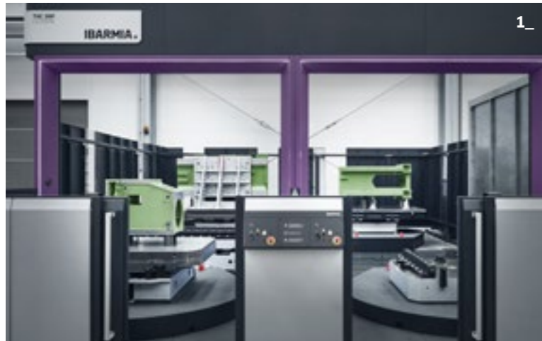
1_ Above, pallet pool with four stations on a THC 30 EXTREME (model with up to \varnothing 3000 mm turning capacity on parts up to h1950 mm and 20t). These rotary stations for loading and unloading parts while the machine is working (2 and 3) eliminate the downtime caused by complex preparations on this type of large-volume parts (see page 21).
